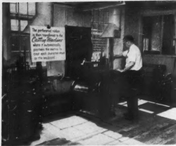
Monotype Caster department in plant of Excelsior Printing Co., North Adams, Mass. The Monotype equipment consists of two keyboards, two casters and one Material Maker. The exhaust hood arrangement draws off melting pot fumes. When this picture was taken, the sun was shining on the impressively clean floor.
